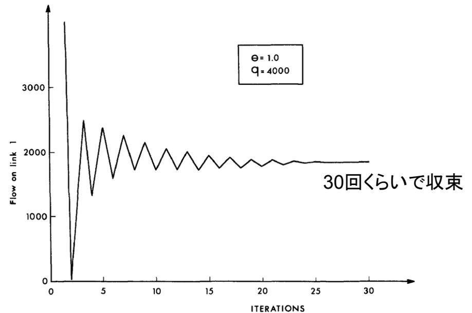
Figure 12.5 Convergence pattern of the MSA for the network in Figure 12.4; the case of relatively large perception variance ( $\theta = 1.0$ ) and relatively high congestion level ( $q = 4000$ ).
