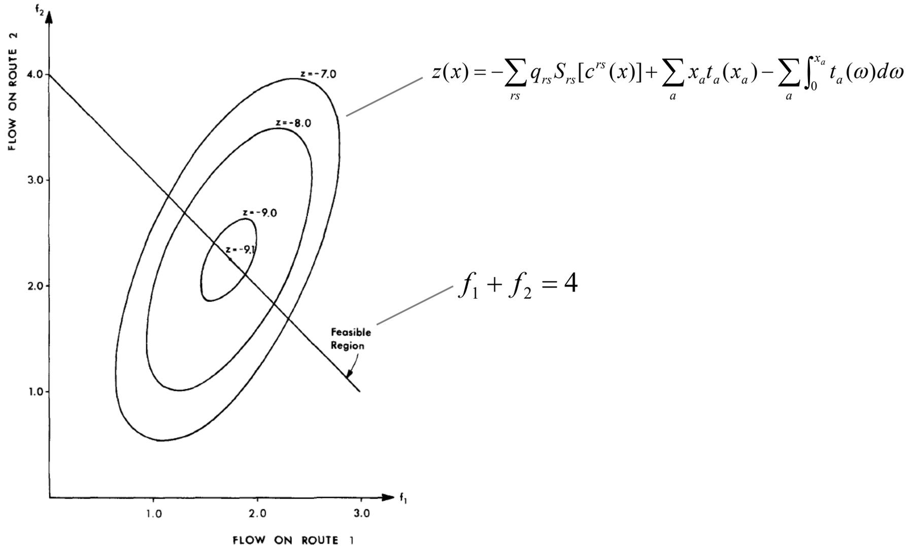
**Figure 12.2** Contour lines of the SUE objective function for the network example in Figure 12.1 (Eq. [12.13] with  $S[c(f)] = -\ln [e^{-c_1(x_1)} + e^{-c_2(x_2)}]$ ). The line shows the locus of points meeting the flow conservation condition. Note that the minimum of the objective function is on the line.
