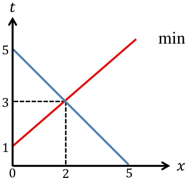
$$\begin{aligned} \min z(x) &= \int_0^x t(\omega) d\omega - \int_0^x D^{-1}(\omega) d\omega \\ &= \int_0^x (1 + \omega) d\omega - \int_0^x (5 - \omega) d\omega \\ &= x^2 - 4x \end{aligned}$$
